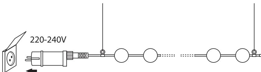
Maximum two sets can be connected together
