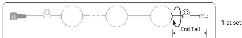
Step 2: Unscrew and remove the lead wire and first ball of the second set.
