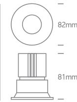
700mA | COB | CCT V | 12W | IP65 | Aluminium
