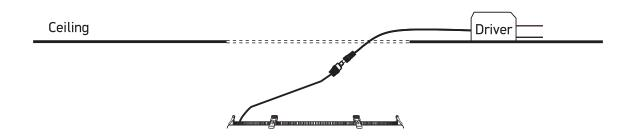
Install fitting using springs supplied.
