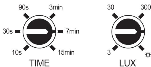
Note: When testing in daylight, please turn LUX knob to ☀ position, otherwise the sensor lamp could not work.
