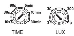
Note: When testing in daylight, please turn LUX knob to -X- position, otherwise the sensor lamp could not work.
