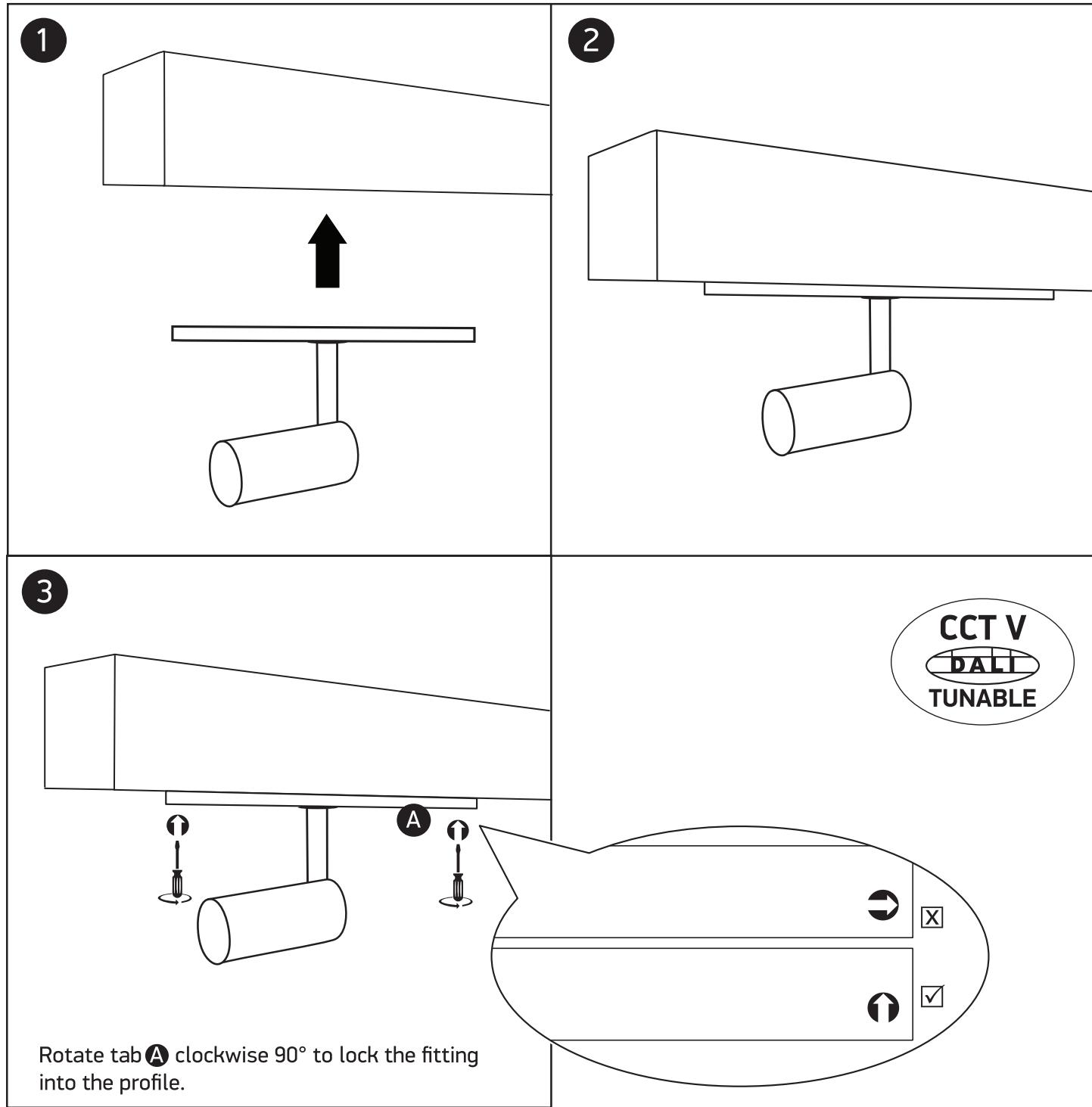
Rotate tab A clockwise 90° to lock the fitting into the profile.
