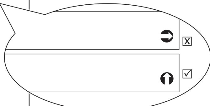
Rotate tab A clockwise 90° to lock the fitting into the profile.
