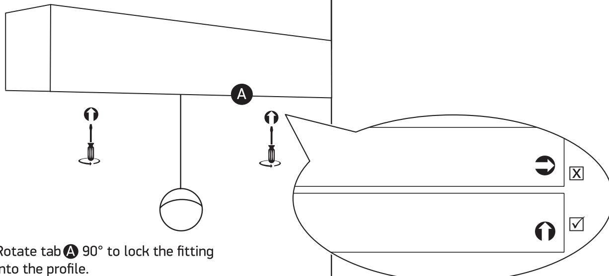
Rotate tab A 90° to lock the fitting into the profile.
