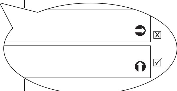
Rotate tab A clockwise 90° to lock the fitting into the profile.
