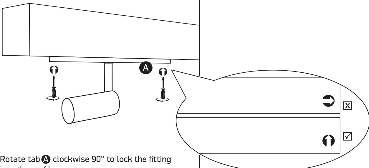
Rotate tab A clockwise 90° to lock the fitting into the profile.
