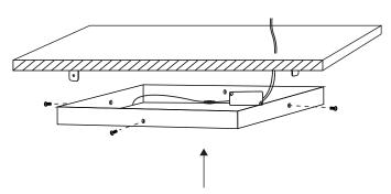
Place the frame on bracket and use screws to fix.
