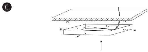
Place the frame on bracket and use screws to fix.
