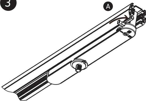
Rotate adaptor lock **A** clockwise 90° to connect the adaptor to the neutral circuit.
