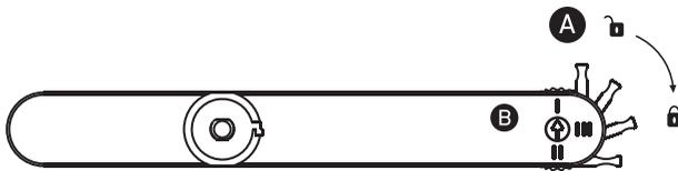
To mount the track adaptor into the track system, first check that the adaptor lock **A** is disengaged.
