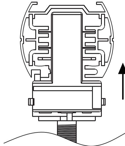
When installing the adaptor into the track, ensure that it is orientated correctly.
