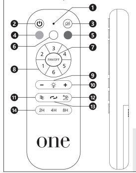
NOTE: To pair a remote to a receiver turn ON the power supply to the fan and press the ON/OFF and MUTE keys on the remote for 3 to 5 seconds. You will hear a beep.
