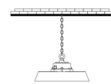
Use a chain, cable, mounting hook, or other mounting hardware to suspend the luminaire. Make sure the mounting hardware is securely attached to a stationary structure and strong enough to safely suspend the luminaire.
