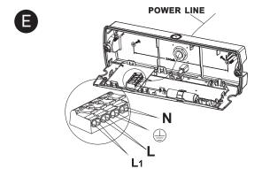
Connect the power line (ensure the power is off) and then insert the battery wires into the PCB. When AC supply is connected, please check if the green LED indicator illuminates to confirm charging of batteries.
