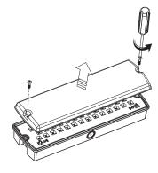
Twist off the two screws and open the diffuser.
