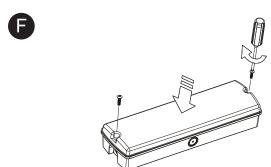
Close the diffuser and then tighten the screws. (Allow a short period for part charging of the batteries and then isolate the mains supply to the fitting in order to check the correct operation of the fitting in emergency mode.
