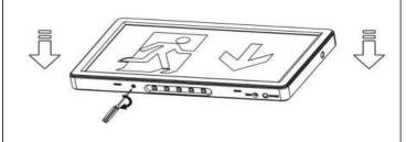
Remove the cover of the emergency. Install it on the wall by using fixing screws. Connect it to the mains supply 230V AC. N⊕ L L1 Check that the green LED indicator is switched on.
