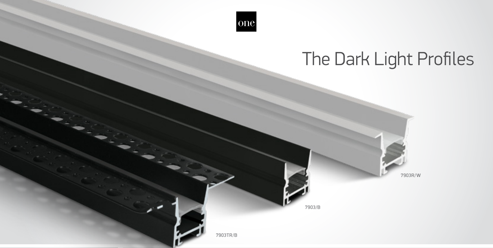
7903R/W | 2m Recessed profile + PC opal diffuser | Aluminium | Suitable for 7820, 7829, 7829A, 7839 & 7843 LED Strips 12mm
