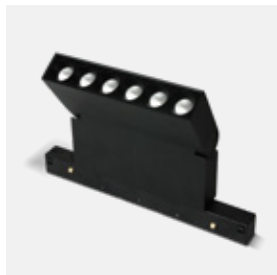
42124BA | 20W | SMD 3030 | Linear spots | Adjustable | Aluminium
