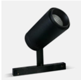
42114CL | 30W | COB LED | DALI | Aluminium
