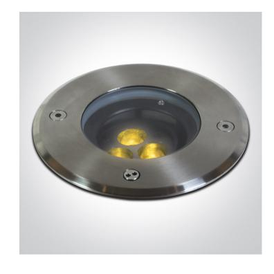
3x1,5W COB LED inground uplight with a 36° beam which is tiltable +/-20°. IP67, stainless steel 316L and die cast aluminium body.
