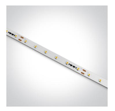
Flexible LED light strip, with SMD2835 LEDs, 60LEDs/meter, 3W/meter.Supplied in 30 meters roll with white PCB and double adhesive tape for a better fixing.
