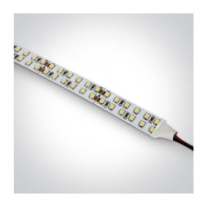
Flexible LED light strip, with SMD3528 LEDs, 240LEDs/meter, 19,2W/meter.Supplied in 5 meters roll with white PCB and double adhesive tape for a better fixing.
