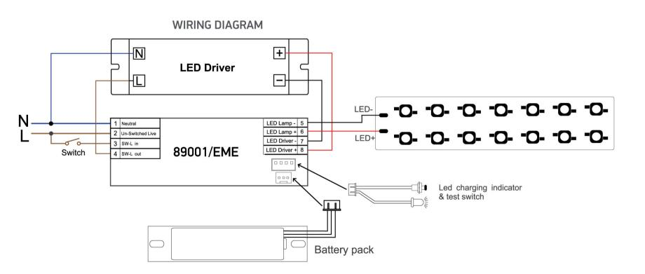
This kit will only operate with LED Fittings/Strips 1-30W suitable for 9-45V DC power supply. The driver automatically adjusts the output LED current to provide the optimum match between the battery and the load, providing maximum illumination whilst ensuring full battery duration.
