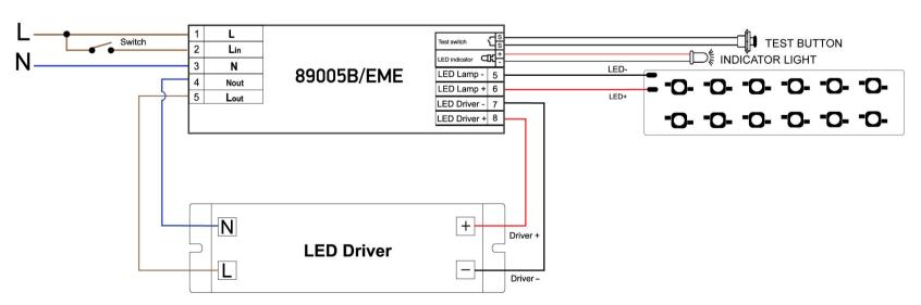
This kit will only operate with LED Fittings/Strips 5-50W suitable for 8-60V DC power supply. The driver automatically adjusts the output LED current to provide the optimum match between the battery and the load, providing maximum illumination whilst ensuring full battery duration.
